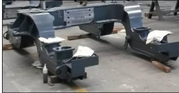
Loco Bogie Frame - Queensland Railways
