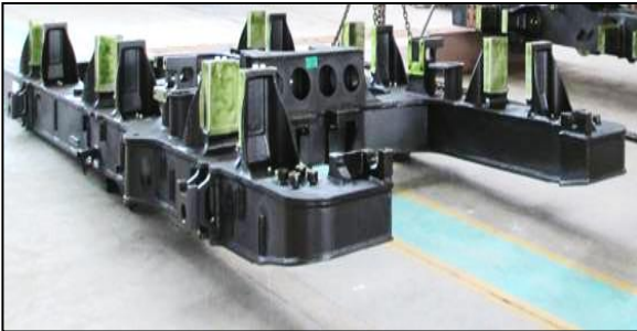
Loco Bogie Frame - Queensland Railways
