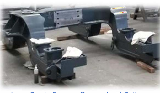
Loco Bogie Frame- Queensland Railways
