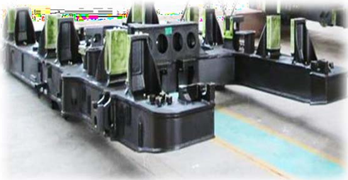
Loco Bogie Frame- Queensland Railways
