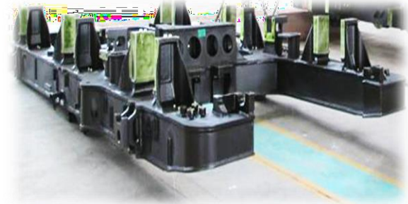
Loco Bogie Frame- Queensland Railways
