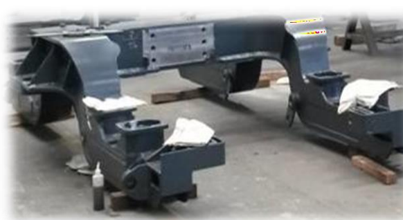
Loco Bogie Frame- Queensland Railways
