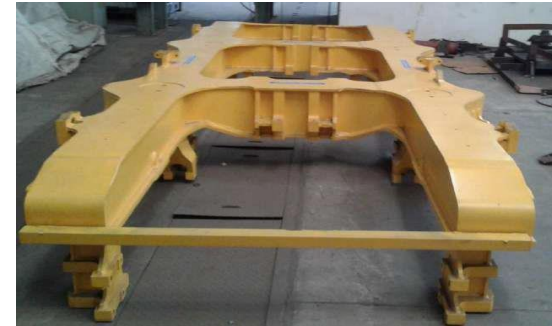
Flexi Curve Loco Bogie- Mozambique
