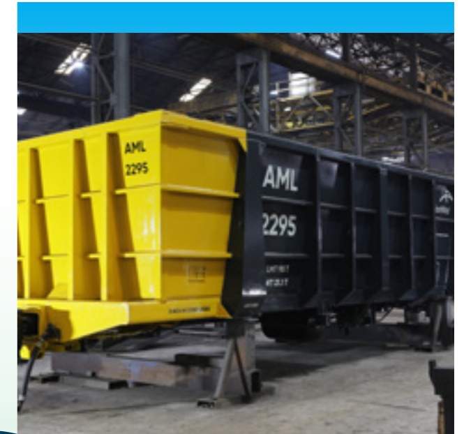
Texmaco designed and manufactured Gondola Wagon Africa, for carrying Iron Ore
