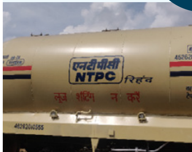
BTAP wagon for carrying alumina and flyash
