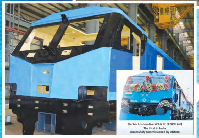
Electric Locomotive Shell for Alstom being manufactured at Sodepur Works.
