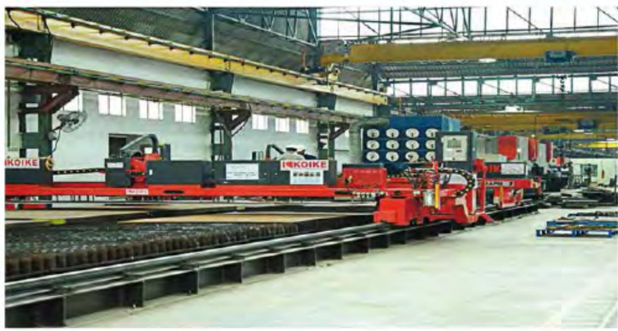
Plasma-Oxy Cutting machine, Koike, Japan
