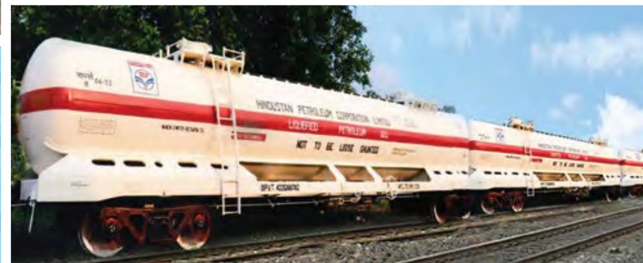
BTPGLN Tank Wagon for transportation of Liquefied Petroleum Gas
