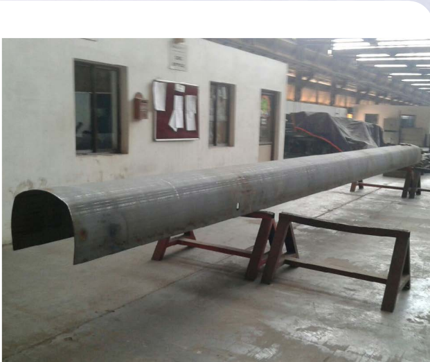
▲ 12 mtr. long Channel Bending
