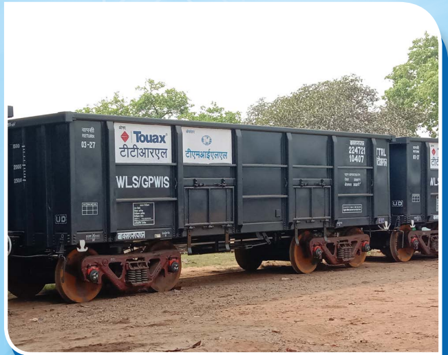
Leased BOXNHL rake for coal carrying
