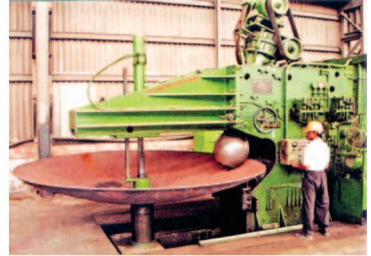
End Dishing Dished Ends 600-4000 mm dia, 5-22 mm plate thickness 50-500 mm knuckle radius
