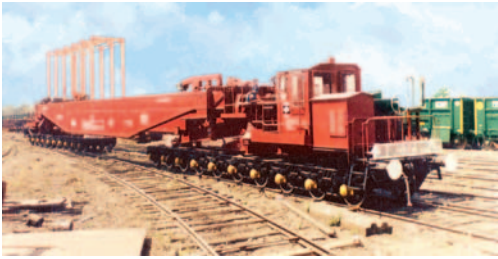
250 Tonnes pay-load car for transportation of Transformers
