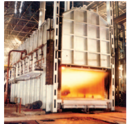
Stress Relieving for jobs up to 19.7 m L x 3.7 m W x 4.38 m H, at centre x 40 t in weight
