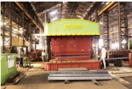
Press Shop 1250 tonnes capacity Hydraulic Press
