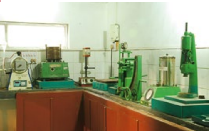
Self Sand Testing Machine, Permeability Meter, Core-Determinater, Sieve Shaker and Clay Testing Machine
